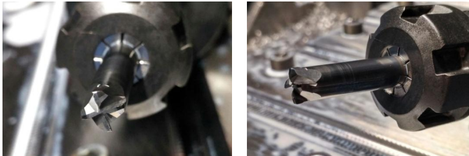
Fig. 6 – Visual identification of the tool wear after process completion.
